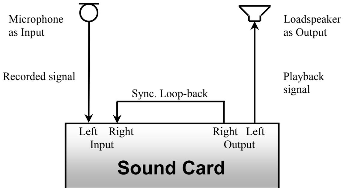
**Figure 3: Schematics 1-channel measurement using feedback loop.**
