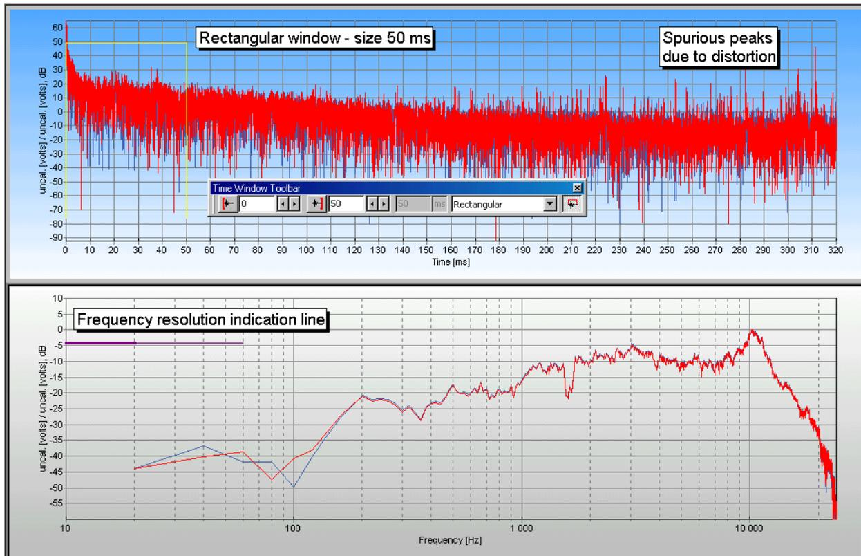
**Figure 3 Multimedia microphone and loudspeaker measured on axis at a distance of ~20 cm. Time window 50 ms.**
