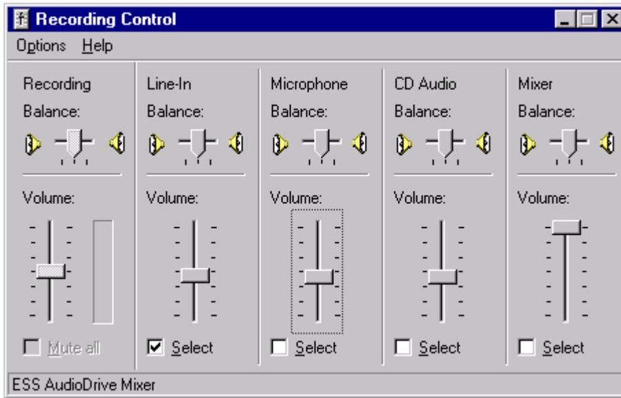
Select the input you would like to use, either line-in or microphone. While you use WinMLS, you probably need to set both the input and output level. You should therefore have one of each open at the same time. To do this, just open a new volume control in addition to the one already open.
