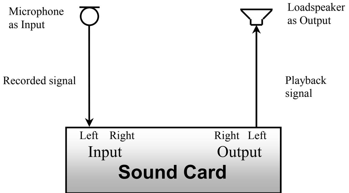
Figure 2: Schematics for one-channel measurement
