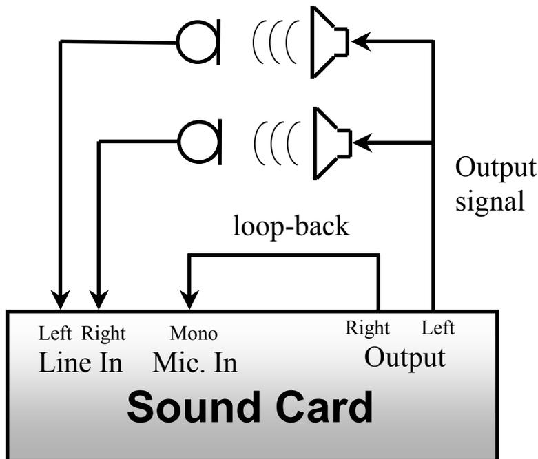
Figure 4: Schematics for two-channel measurement using synchronization loop-back for two physical inputs.
