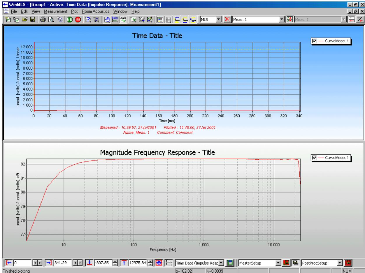
**Figure 1 Screenshot after loop-back measuring the Digigram VX222 sound card.**
