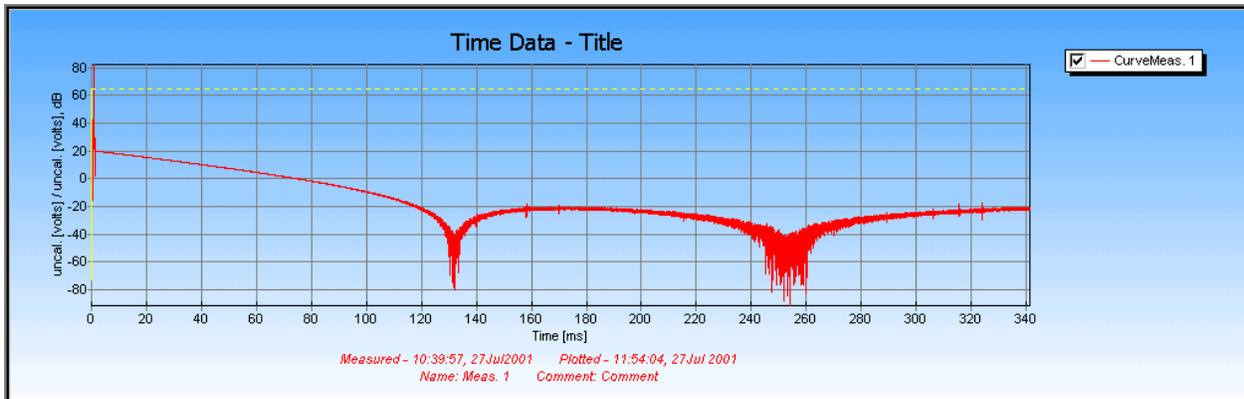
**Figure 2 VX222 sound card measured loop-back, plotted using dB as y-axis.**
