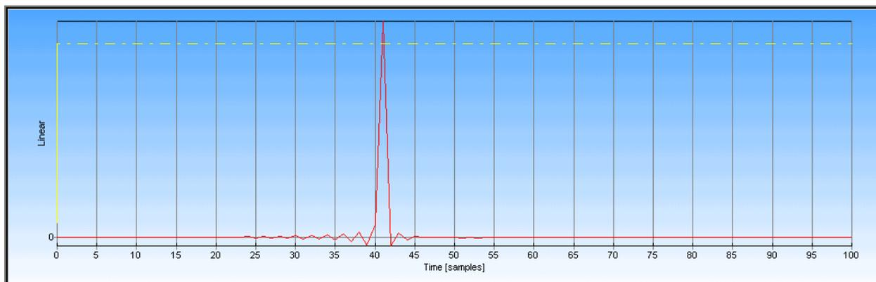
From this we see that the sound card has a delay of 41 samples. It is possible to correct for this delay, how to do this is explained in the measurement part of the FAQ.
