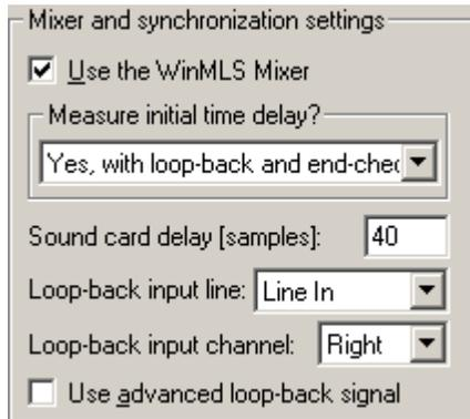
Now select the **Loop-back Input Line** you used for connecting the loop-back to, in the figure above **Line-In** is chosen. Make sure **Loop-back input channel** is set to **Right**. The sound card delay must now be set in samples, this we already have found in the first measurement procedure we described. This number can vary from 10-80. After typing this number, click OK to exit the dialog box.
