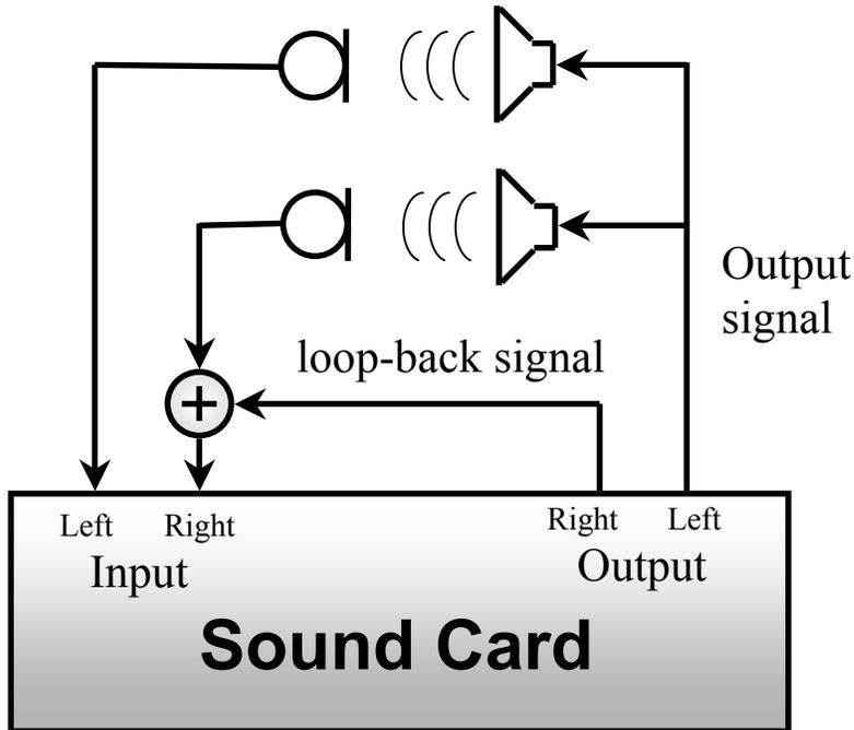
**Figure 3: Schematics for two-channel measurement using synchronization loop-back for one single input.**
