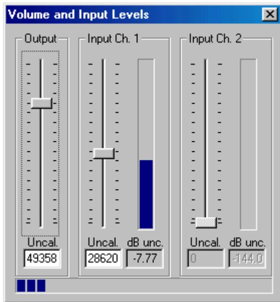
The input level must be less than zero to avoid clipping, but as near zero as possible. In the figure, the input level is  $-6.51$  dB, which tells how far it is from clipping. If the level is lower than  $-40$  dB or increasing the volume does not increase the level, the cables are not properly connected.
