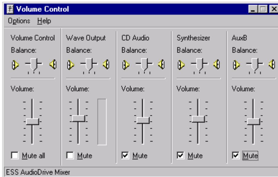
The volume control above shows the output volume. When using WinMLS you only use the **Wave Output** shown in the figure above. It is a good idea to mute the other possibilities as shown in the figure above. But do not mute the master **Volume Control**.
