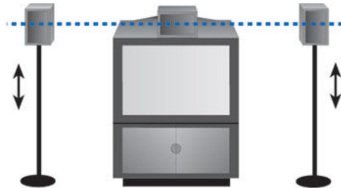
Figure 7: Adjustable stands for the left and right speakers can make it easier to achieve the same height as the center speaker.
